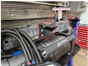
4. Place grill support on top of grill support brackets and fit 6 x M6 bolts washers and flange nuts but don't tighten. Tighten support bracket to Radiator support first then tighten grill support panel bolts. Attach Grill clip housing on top of grill panel and fit 4 x M6 bolts washers and nuts.
