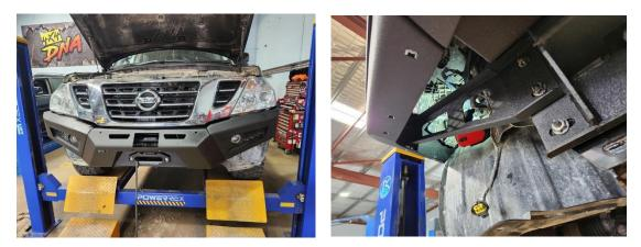
9. Drill 2 or 4 holes (depending on model) for park sensors. The holes need to be 26mm diameter and placed as shown in picture. Refit Park sensor loom removed from factory bar. Note May need to extend sensor looms by cutting and soldering extensions into the 2 wire sensor looms. Fit park sensor bezels removed from factory bar and fit park sensors. Connect all sensors and cable tie loom to secure.
