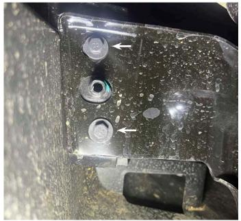
6. Carefully remove the 2 plastic covers on the front of the bar and remove the 2 bolts behind the cover
