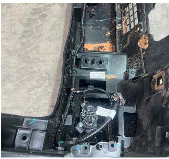
12. Remove the parking sensors from factory bar and retain. Make a note of position and orientation of sensors and match when refitting to bullbar
