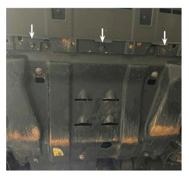
2. Remove the bolt and screw from the bottom outer sides of the bar
