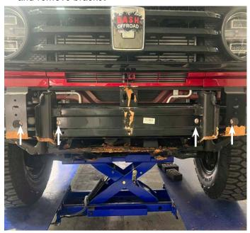
9. Remove the 5 bolts in chassis brackets and remove brackets
