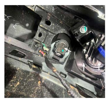
13. Carefully remove the parking sensor mounts with a scraper or similar, these are held in with double sided tape. Make a note of position and orientation of sensors and match when refitting to bullbar
