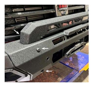
25. Bolt the ends of the bullbar to the wing support brackets with 2x M10 x 25mm bolts and washers. Leave these finger tight. Align the ends of the bullbar with the guard and wheel flare and then tighten all the wing support bolts
