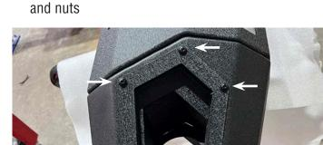
17. Fit the fog light insets with M6 button head bolts
