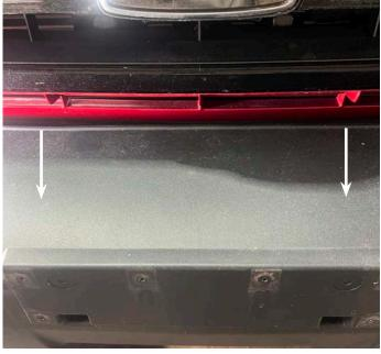
9. Remove the 4 bolts in the bumper support bracket and remove bracket
