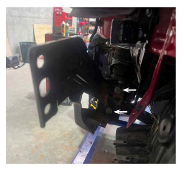
11. Unplug and remove the wiring loom from the factory bar and retail loom
