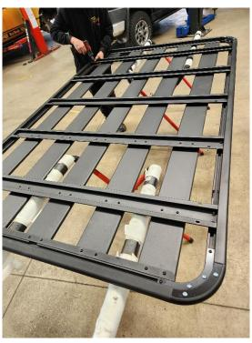
4. Attach wind deflector by inserting 4 x M6 channel nuts into front rail of roof rack (any end you like) Place wind deflector and align channel nuts as required. Fit 4 M6x12 hex bolts loosely. Centre wind deflector and tighten bolts.
