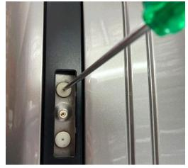
TIL Models will need to remove the factory roof rails. The trim over the centre mounting point will need to be trimmed using a small pair of tin snips as shown. Mark and cut Centre mounting trim towards the rear of the vehicle and extend the opening by 55mm long. To expose the second mounting hole.
