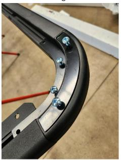
2. Fit M6 channel nuts and slide along to line up with holes in the inner corner supports and fit 8 M6 x 12mm hex head bolts to each corner but don't tighten yet. Place 5 long platform rails one at a time under frame and align holes in ends and fit M6 x 15mm hex head bolts loosely into each end.
