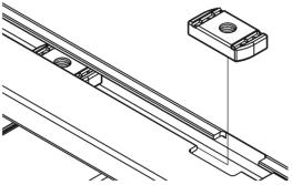
Place Grab Handles (1) on your platform, securing to channel nuts using M8 Screws (2), Spring and Flat Washers (3 & 4), ensuring they are fully tightened
