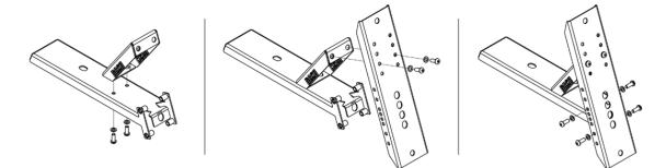
2. From MAXTRAX Pin Kit (not included) fix Mounting Pins, M10 Flat Washers, and Nyloc Nuts to both Brackets, ensuring pins are oriented as per cover image
