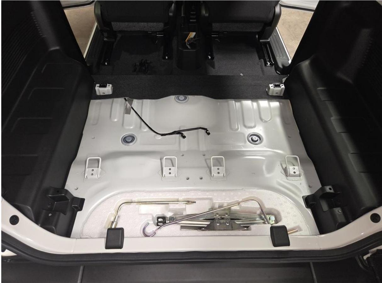
7. Remove the 2 black plastic retaining clips by carefully levering in the 4 tabs using a small screw driver or similar.
