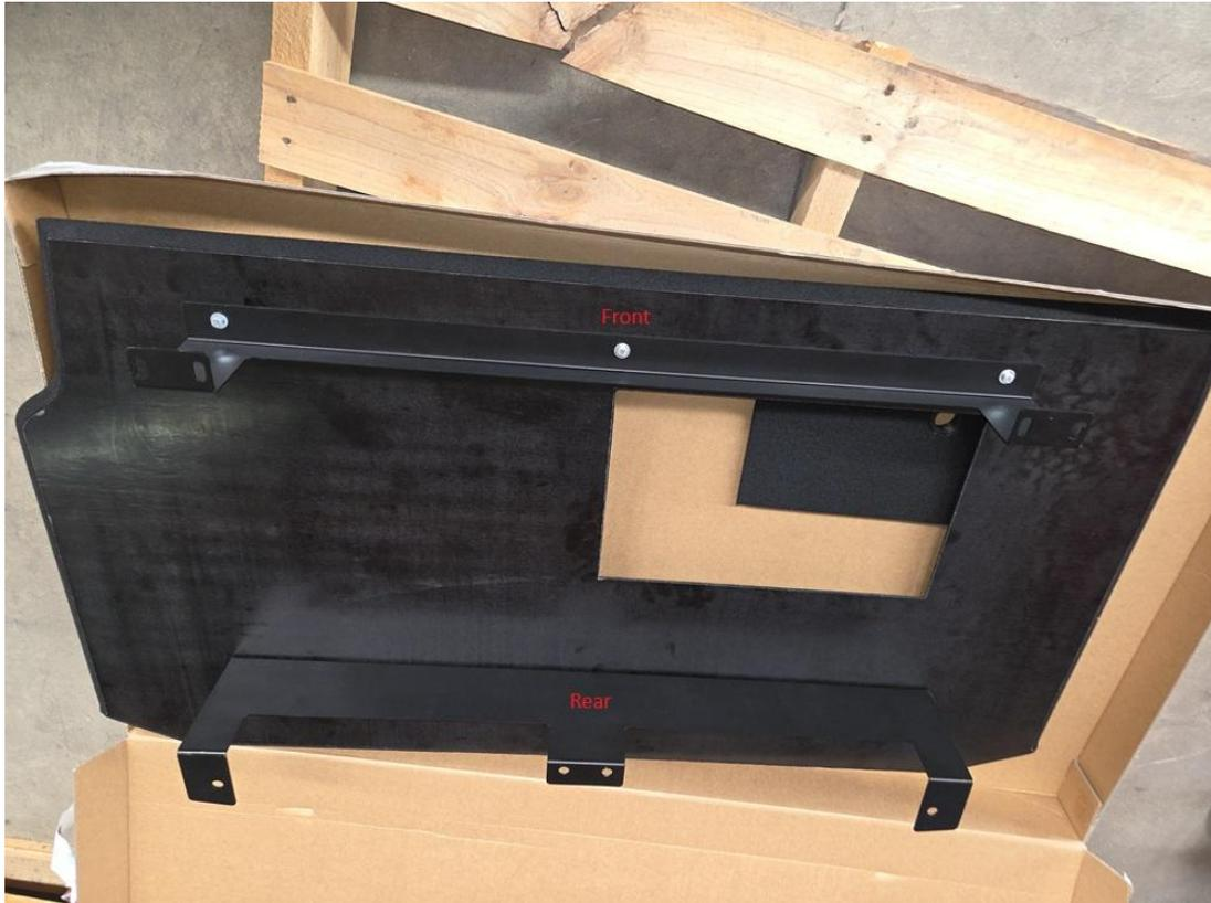
9. Lift the DASH False Floor into place. you will have to lift it in at an angle, placing the passenger side down first to clear the 12-volt accessory socket.
