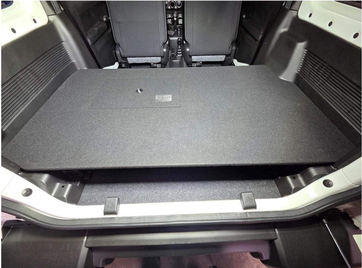
1. Remove the rear storage tray. Lift the lid and gently pull straight up.
