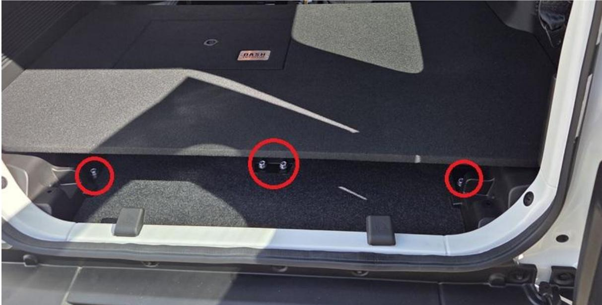
11. Fit the bolts and flange nuts to the front support brackets as shown. Hold the nuts under the bracket and screw in the bolts and washers on both sides.
