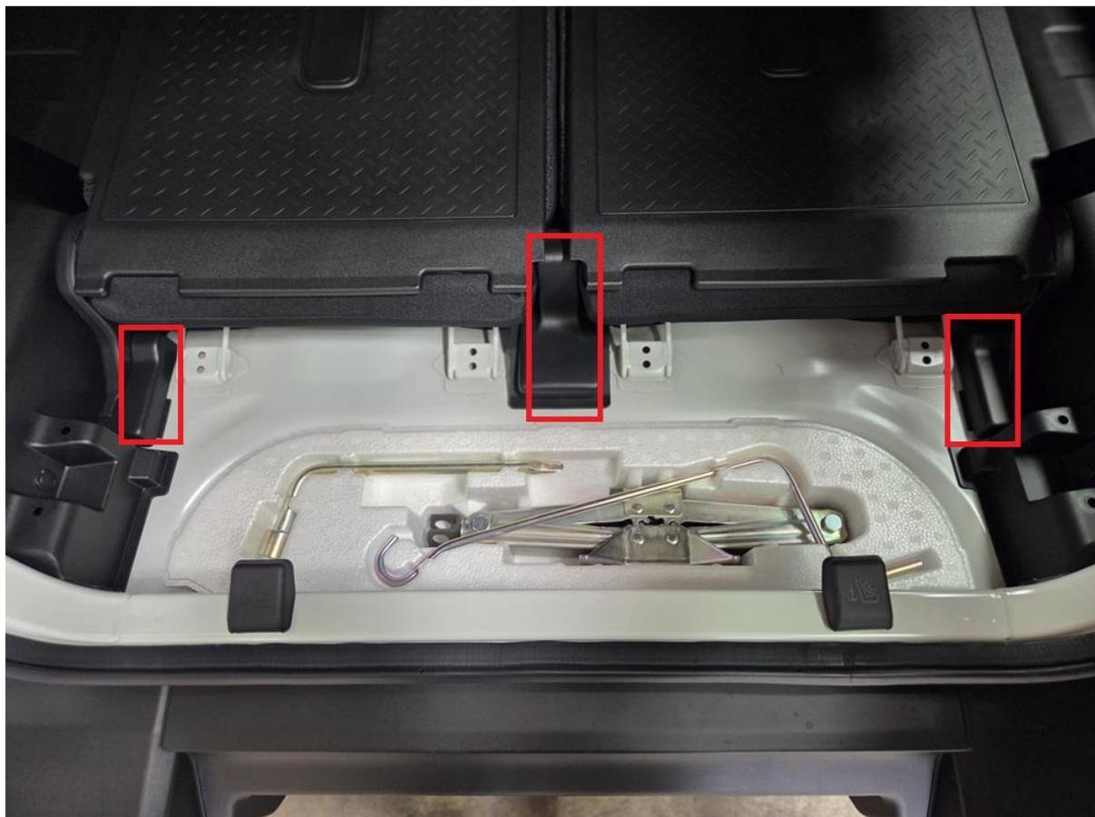
3. Remove the 4 14mm bolts holding the seats down.
