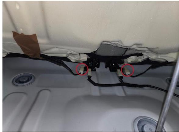
5. Remove the centre bracket trim to access the bolts and remove the 4 14mm bolts holding the seats down. Remove the 2 14mm nuts attaching the seatbelts to the side brackets. Unplug the seatbelt sensor connectors.
